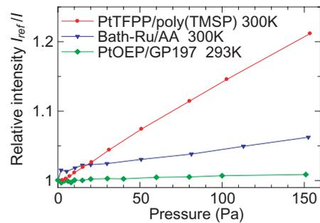
Fig. 8 Stern-Volmer Plots (発光強度の圧力依存性)
